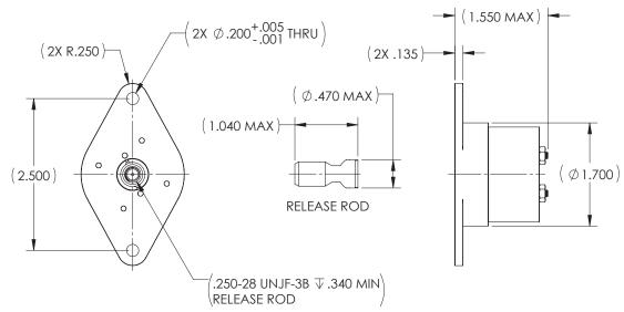
Note: Model 9102G Release Mechanism shown. Different configurations available with alternate release rods, mounting features, and connectors. Metric configurations are also available.
